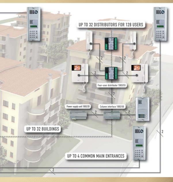
A system for a new block of flats can be made using the dedicated 2Voice wire 1083/90 or 1083/92. Existing wires can be used when modernising an existing system. Refer to the wire table on page 37 for limitations concerning number of users, distances and extensions.
